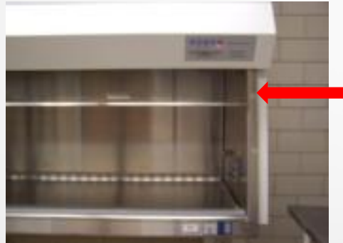
SASH TOO HIGH
